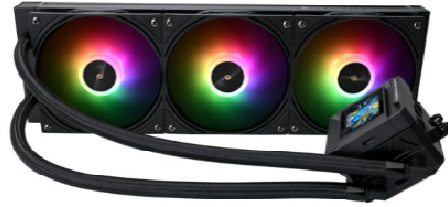
利民 (Thermal Right)水冷泵 (三相无刷ACM6753/ACM6732)
